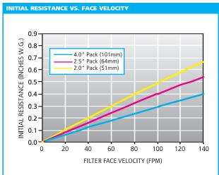
Note: This graph represents a typical rating. The inside face dimension (not including filter frame) is used to calculate resistance. Filters are tested at 100 fpm at the factory. Recommended service resistance is approximately two times the initial resistance at the factory test.
